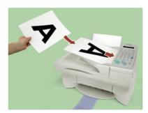
**Document glass:** Place the original face down on the glass with the top edge against the document guide. Make sure the center of the original is aligned with the center mark on the document guide.
